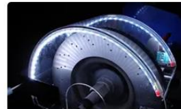
Chip protection cover A cover with LED helps preventing chips from flying and enables precise work
