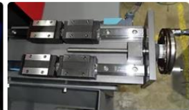
LM guide rail Linear Motion guide rail keeps high precision even with long term use
